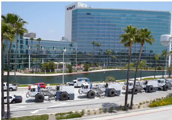
A four-truck seismic fleet sourced on Shoreline Drive and other city streets in Long Beach as part of a 3D seismic survey for Signal Hill Petroleum Inc. Image courtesy of NodalSeismic.
